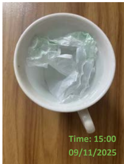
Fig. 28: Bioplastic immediately after soaking
