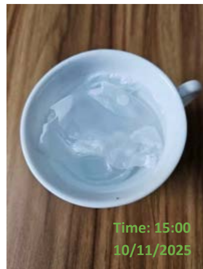
Fig. 29: Bioplastic after soaking for 24 hours
