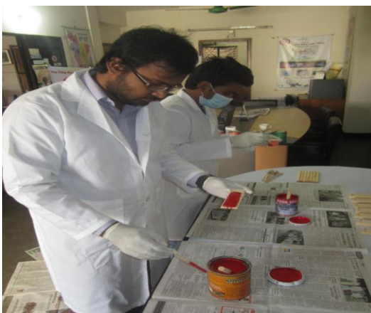
Application of the paints to wood pieces and drying of the painted woods
