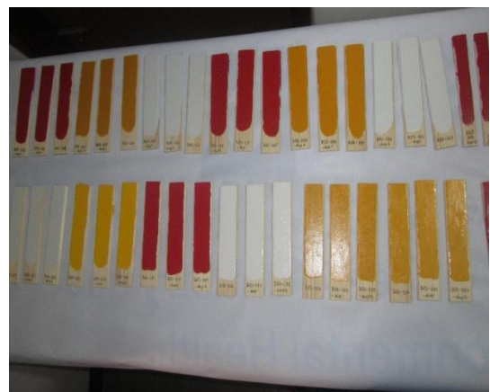
Application of the paints to wood pieces and drying of the painted woods
