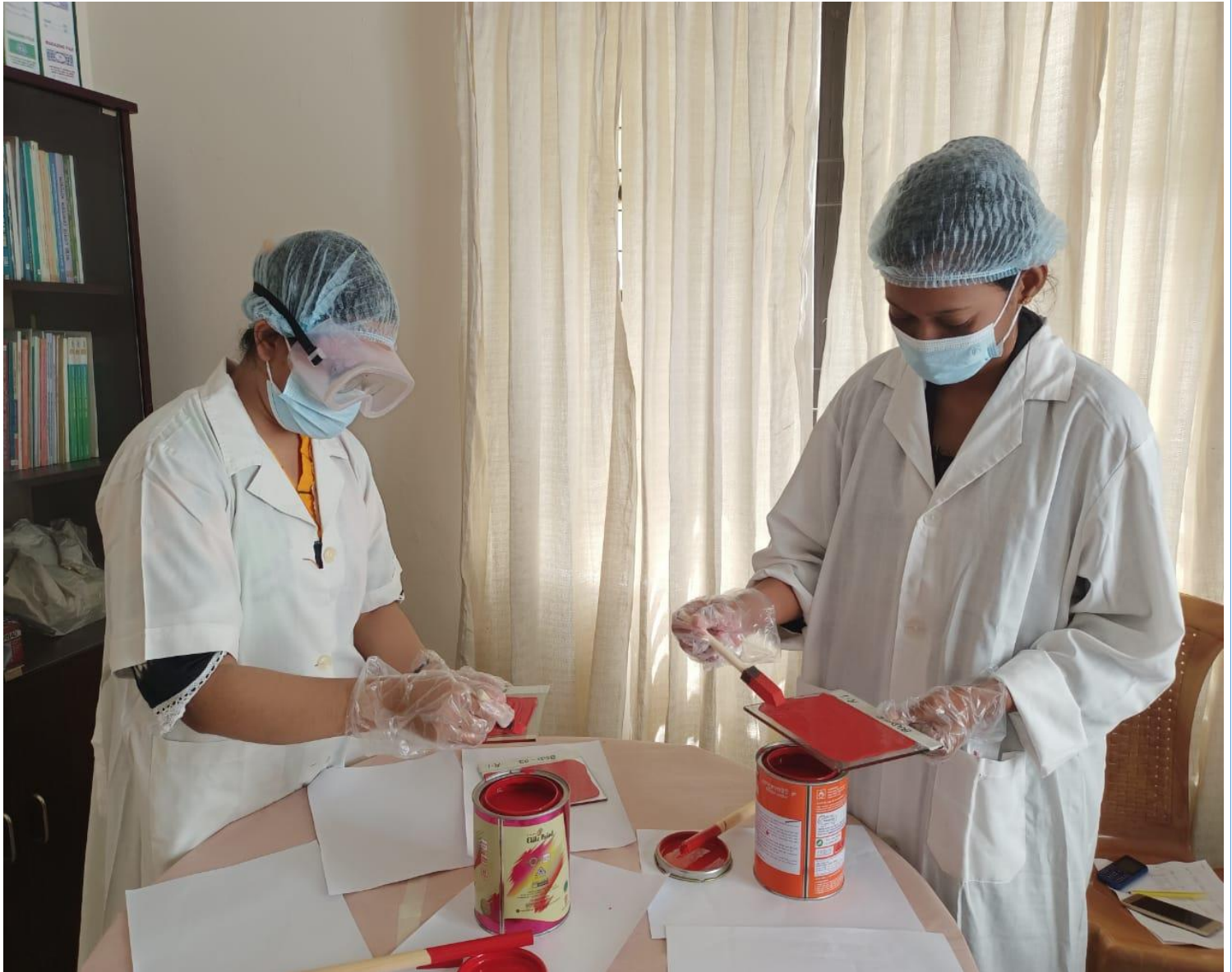
Figure 4: Paint Sampling in Glass Slide
